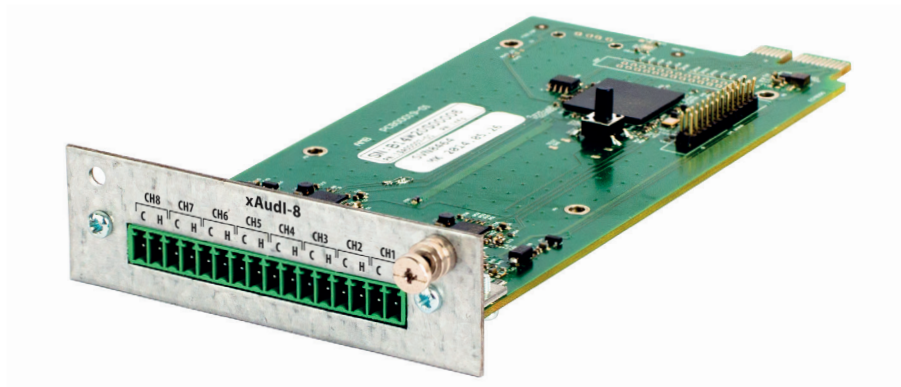
Drawing 29. 8 audio input card
