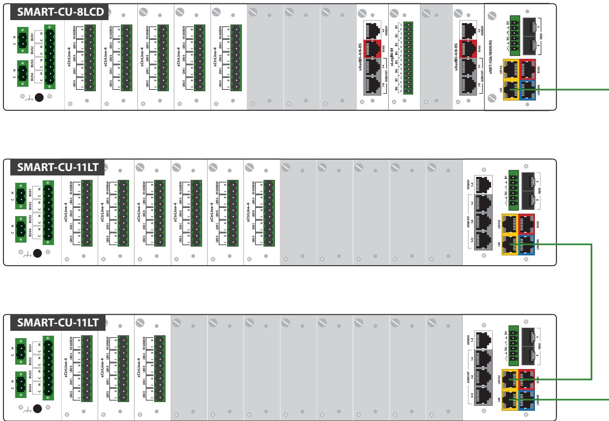
Drawing 72. Example of connection of control units in daisy chain topology
