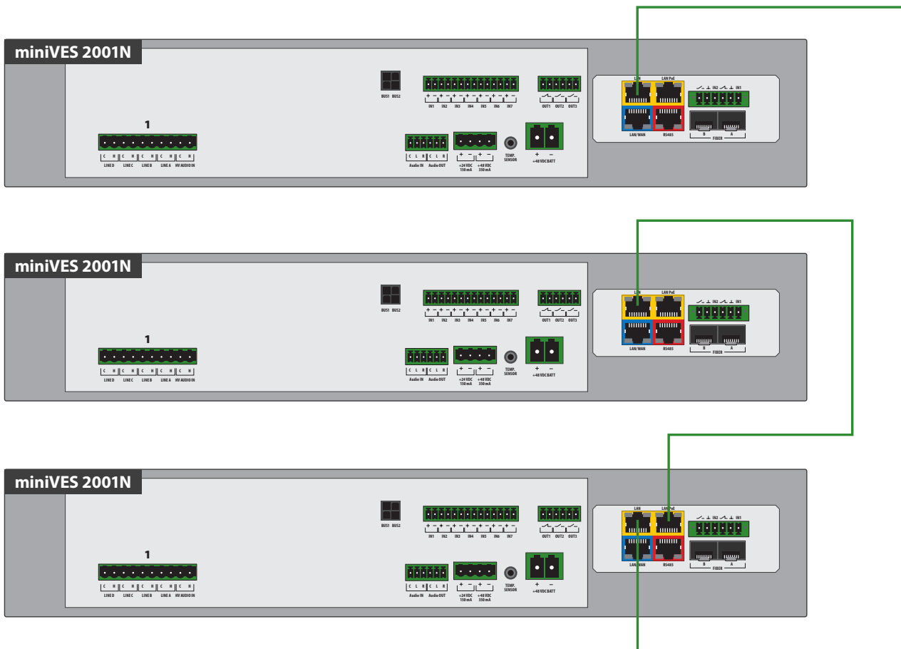
Drawing 64. Example of CHAIN topology control units connection
